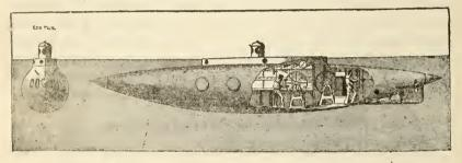
SUBMARINE BOAT WORKING BY ELECTRIC POWER.
